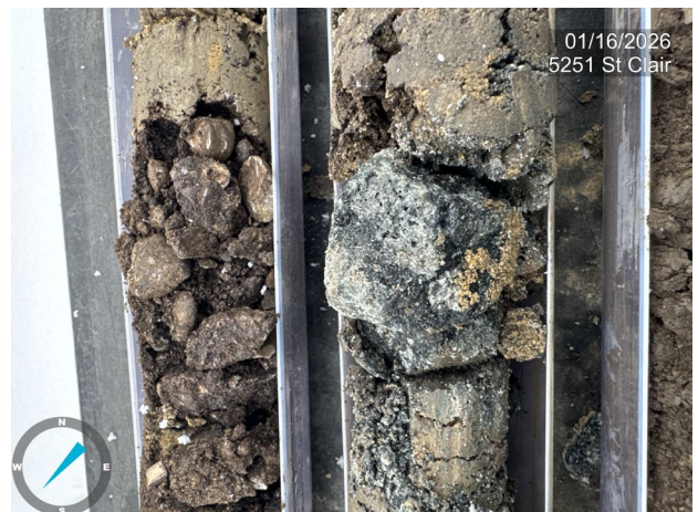
Photo 6: View of the slag at 3' bgs in 5251 SB-02.
