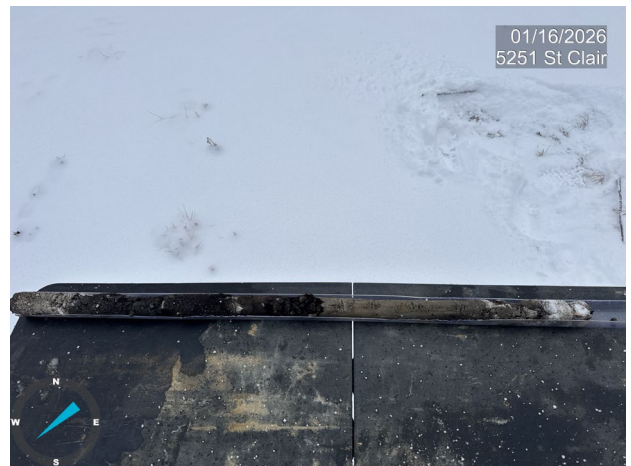
Photo 4: Viewing soil recovery from 5251 SB-01, facing southwest.
