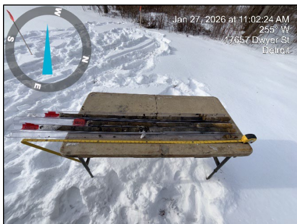
Photo 5: Viewing 17657 SB01, SB02, SB03 soil recovery, facing west.
